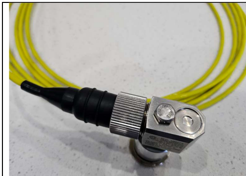
Accelerometer w/ weatherproof cable
